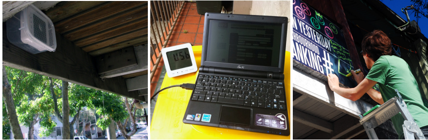
Fig. 3. Left: Hidden storage of a separate electricity monitor allowing uninterrupted access to the data. Center: Netbook and electricity monitor used for downloading and updating displays. Right: The manual update of the daily neighborhood ranking using a ladder.
